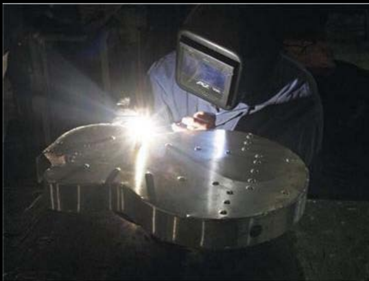
Kari Konchalski welds the seams of one of Jim Normandy's arch top aluminum guitars at Zephyr Engineering
